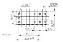
\*) With the recommended PCB hole sizes a grid pattern from 2.5mm to 2.54mm can be used.
